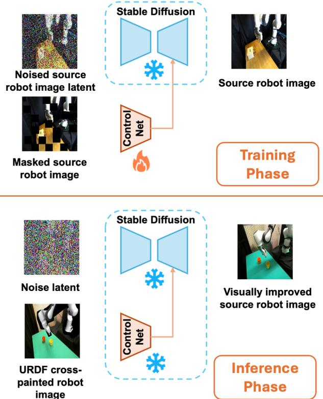
Fig. 7: Robot cross-painting with diffusion generation. We utilize a ControlNet to transfer the pre-trained Stable Diffusion into the robotics domain. The upper part presents the training phase, in which we finetune the parameters of ControlNet while keeping the Stable Diffusion frozen using a masked reconstruction objective. The bottom part presents the inference phase, where a URDF.
