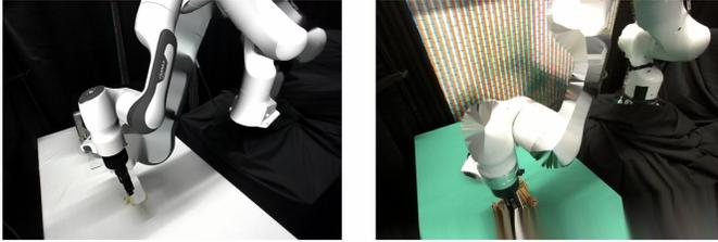
(a) Example of Camera Calibration Error (b) Example of Camera Reprojection with Large Pose Differences
