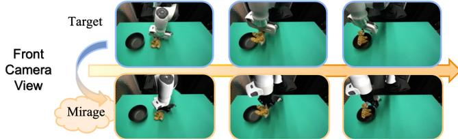
Fig. 6: The front camera angle in the 2-camera experiment in Table IV. **Top:** The actual observations of the target robot during the rollout; **Bottom:** the cross-painted images generated by Mirage.
