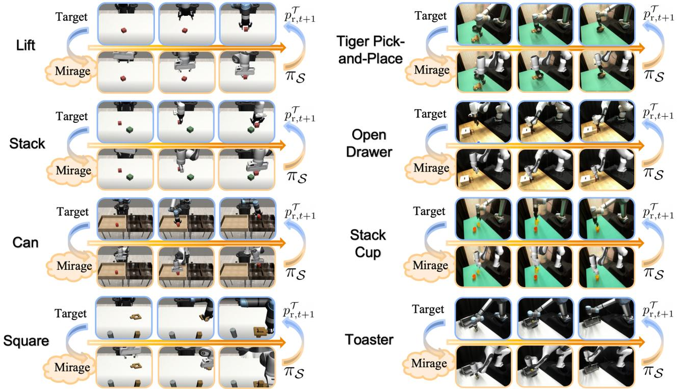
Fig. 4: **Trajectory Rollouts of Simulated (Left) and Real (Right) Tasks.** For each task, the top row shows the actual observations of the target robot during the trajectory rollout, and the bottom row shows the cross-painted images generated by Mirage that are passed to the source robot policy  $\pi_S$  to obtain the desired target robot pose  $p_{r,t+1}^T$ .
